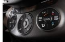
Climate control (HVAC)
